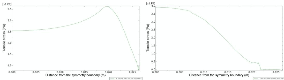
Figure 8: Sizes of developing and steady state fracture process zone
