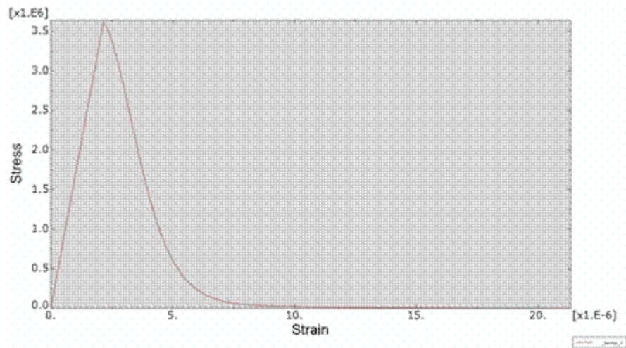
Figure 5: Stress-strain/elongation relation of the cohesive element
