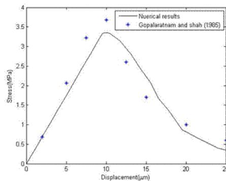
Figure 6: Stress-displacement curve of the concrete specimen and comparison with experimental results
