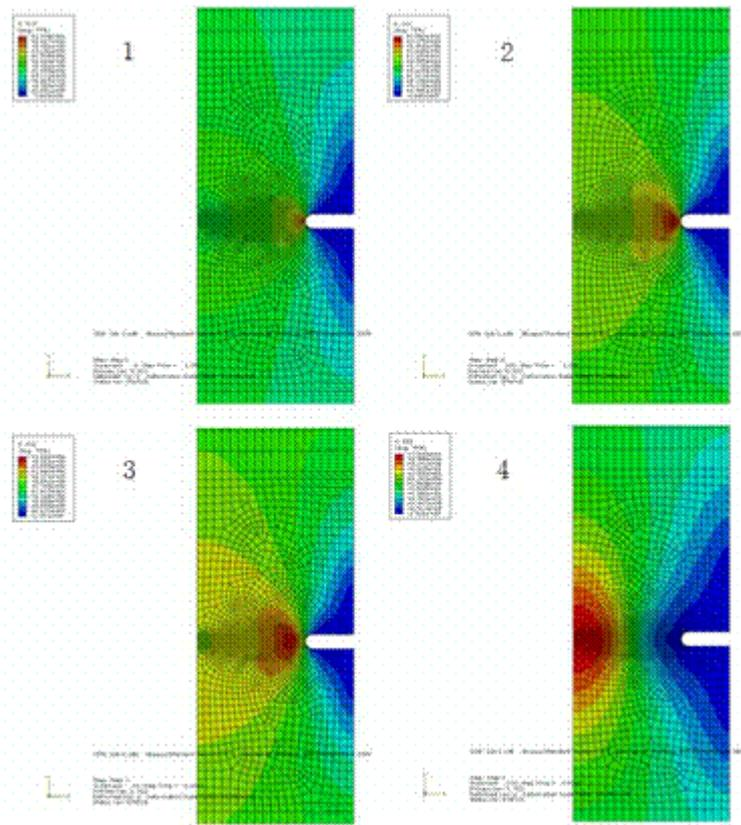
Figure 7: Tensile stress contour (S22) around the cohesive interface at different loading level
