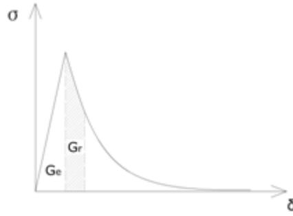
Figure 3: Illustration of various energy release rates
