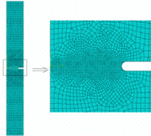
Figure 4: Element meshes of the whole specimen and near the cohesive interface
