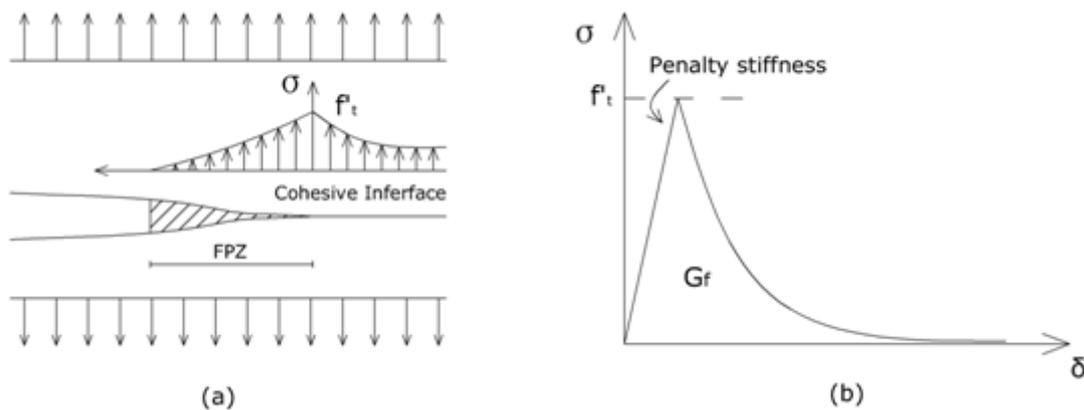
Figure 1: (a) Schematic of mechanism of cohesive interface (b) exponential softening traction-separation curve for cohesive material
