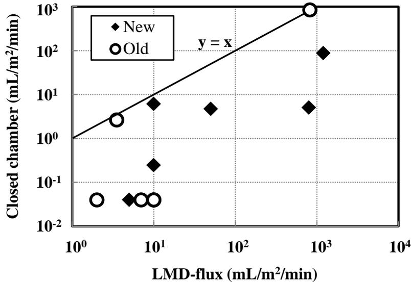
**Figure 3: Relationship of methane gas flux between simplified method and closed chamber method**
