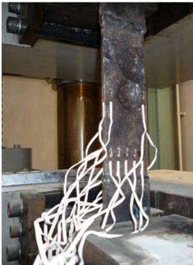
Figure 4: Specimen prepared for the tensile test
