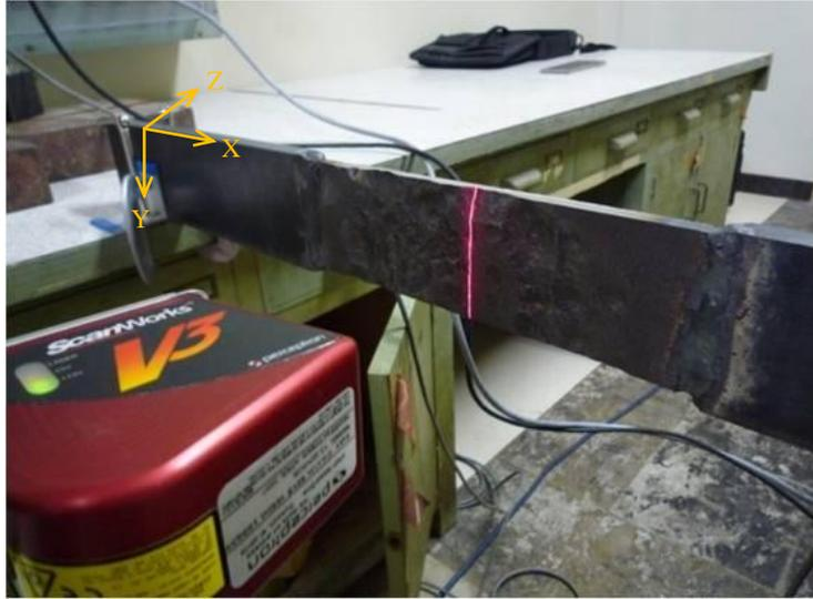
Figure 2: Condition of thickness measurement
