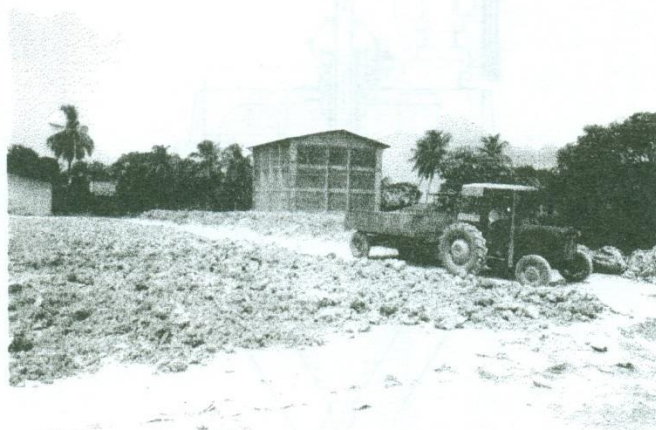
Fig 7. Solar drying of ball clay using the paved area
