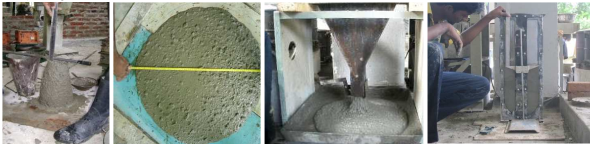
Normal concrete: Slump test Self-compacting concrete Slump flow test Self-Compacting concrete V Funnel test Self-compacting concrete U-Box test
