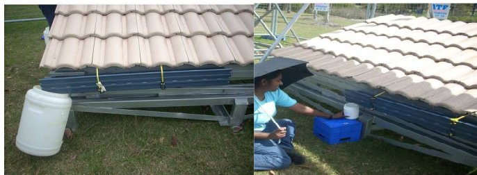
Figure 3 Collection of a) pollutant build-up samples; b) Wash-off samples
